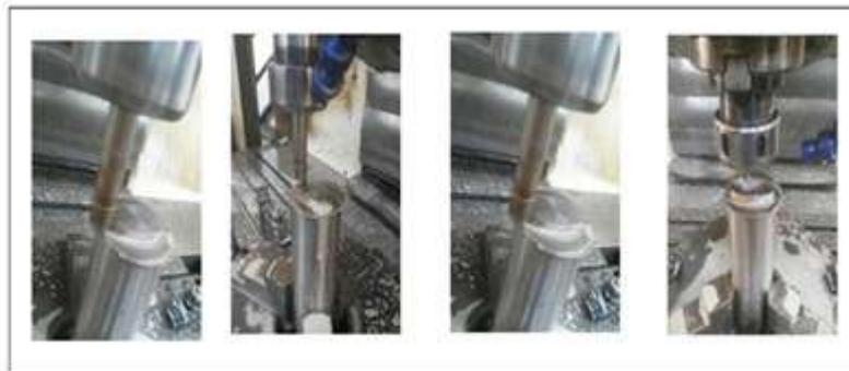
**Figure (5):** Photographic of ribs machining processes
